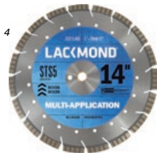
4. D-1 STS-5 SERIES - DIAMOND SAW BLADE: Castellated segmented turbo rim for aggressive and precise cuts. .575" fully impregnated raker, undercut protection segments to prevent knife-edging in abrasive materials, .350" usable diamond depth. Air-cooling core for heat dissipation. Slanted core design for maximum cutting speed. Pre & post tensioned core to eliminate loss of tension. Available in 4" - 24" Diameters. Applications include: cured concrete, green concrete, asphalt, block, stone, granite, piling, overlay, brick & block combination and more. Suitable for: hand saw, hand held high speed saw, low horsepower walk-behind and masonry saws. — PREMIUM SERIES! • Economy blades available. • We can find your blade for less money. • Please specify size for price.
