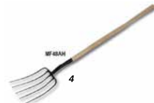
4. H-14 TOUGH-DUTY FORGED MANURE FORK: 5 oval tines, 12 1/2" long, 9 1/2" spread at points. One-piece forged head. 8" ferrule w/ cap. 54" lacquered ash handle. • 5 Tine • 6 Tine
